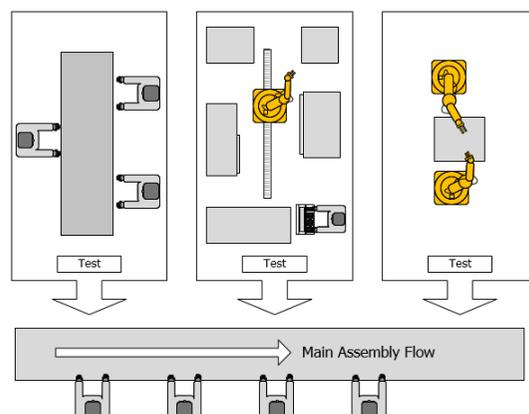
Figure 6: Main Line and Feeding Pre-assemblies
