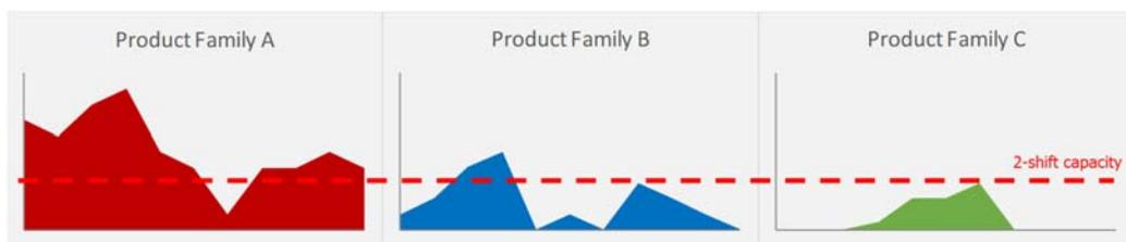
Figure 7: Demand and Capacity (Dotted in red) for the Three Dedicated Assembly Lines
